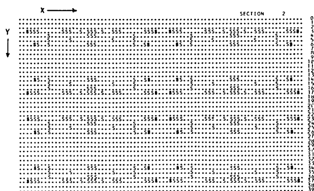
Fig. 2. This section of the B_8Cl_8 symmetry map was calculated with a threshold value of 100 in the Patterson map. Darkened positions indicate the choices for the first tentative atom position which would be consistent with the refined chlorine positions.
